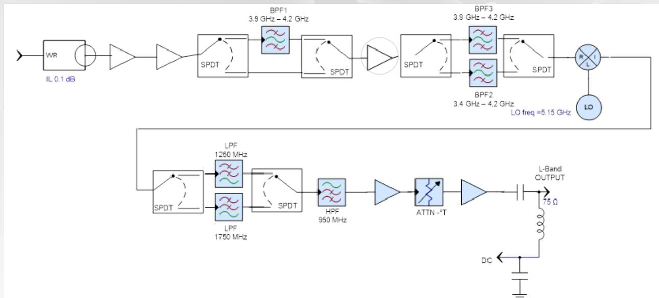
**Figure 2: Norsat 3200-sBPF Simplified Block Diagram**
